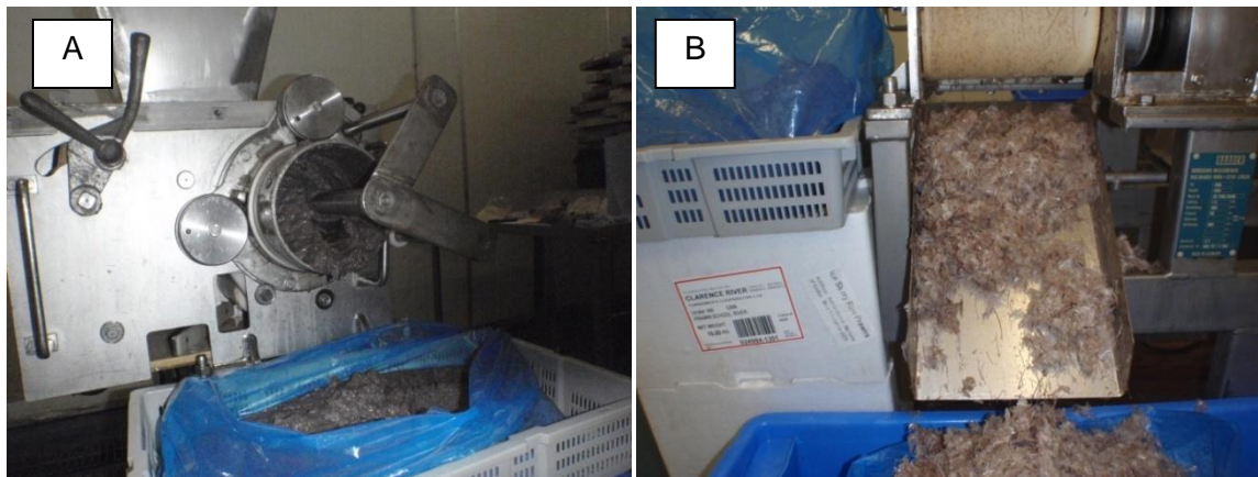
Figure 3 Baader separator during processing of green chilled prawns (Trial 2); (A) collection of the extracted prawn meat, (B) collection of the shell
